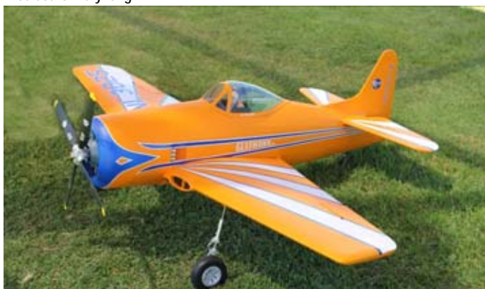
A Grumman F8F Bearcat by Shane Orchard. This model is 1/7 scale, spans 1.5m, and is electric powered.
