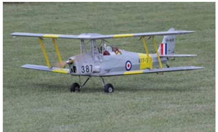
Tim de Haan's Tiger Moth is an ARF by Austar. Wingspan is 2m and it's powered by a Saito FG20 four stroke engine.
