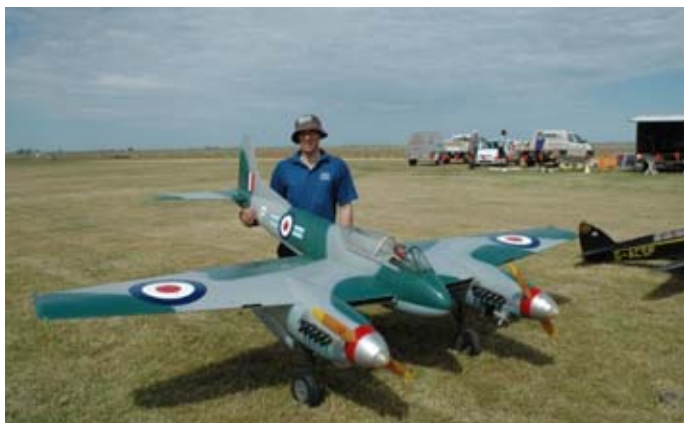
Richard Mudge with his DH.103 Hornet powered by two DJ 80 engines.
