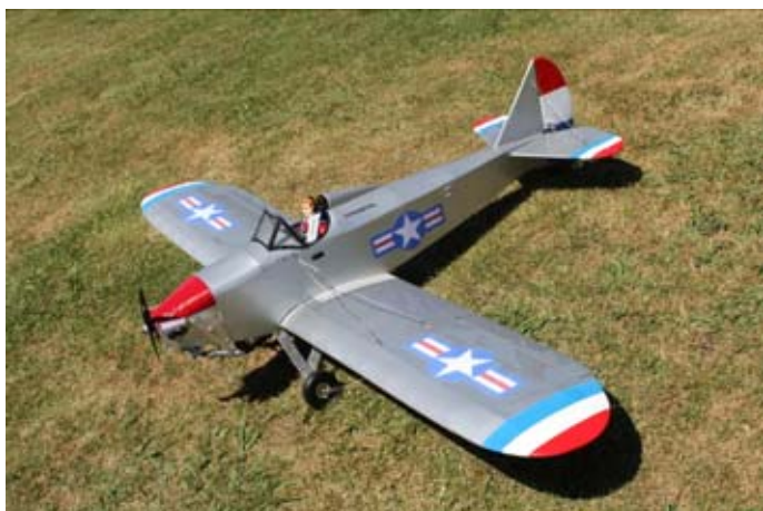
Greg Mitchell's Bowers Fly Baby has been redecorated since last year and now sports stars and bars. Model spans 2m and is powered by a Saito 80 four stroke engine.
