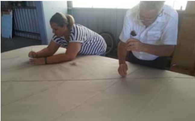
Stitching the fabric to the ribs. thirty stitches per rib, twelve ribs per wing. Again note the seam at 45 degrees – this 'bias' gives additional strength and assists with the wing returning to neutral after warping.
