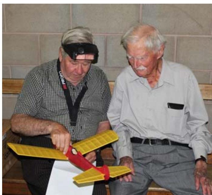
Reg Register and Jim Fullarton discussing Reg's half size replica "Sportster" designed by Jim and published in "Aircraft" magazine in 1950. The model is 0.58m wingspan and electric powered with radio controlled motor, elevator and rudder. The electric drive motor is concealed inside a half scale replica of the Mills 1.3cc diesel engine.
