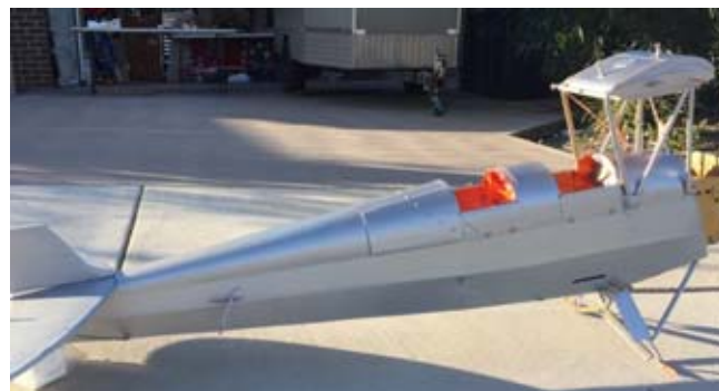
Silver base coat applied to the fuselage.
