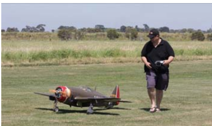
Mario Schembri with his P-47 Thunderbolt. Built from the Zirola plan, the model has a wingspan of 2.3m and is powered by a Zenoah 62cc petrol engine.
