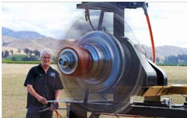
Tony Wytenburg of CAMS running the first reproduction rotary engine at Omaka NZ.
