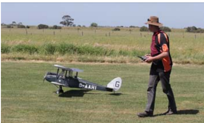
Rob Popelier came from Shepparton with his DH 60 Gypsy Moth. The model is 1/4 scale with a wingspan of 2.3m and is powered by an OS 120 four stroke engine.
