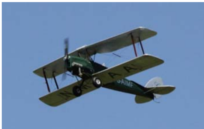
Ian Farrar's DH. 82 Tiger Moth is 1/6 scale. Wingspan is 1.4m and it's powered by a RCGF 15cc petrol engine.
