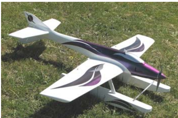
Tony Gyoles "Sea-E-Dart" is all composite and electric powered. It's fast and slippery in the air and handles very well on the water. Kits are available from Tony, mob: 04193-04193.
