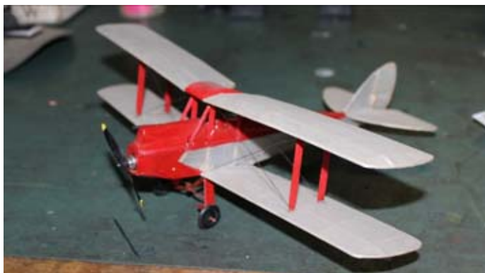
Reg Register's Peanut Scale DH. Gypsy Moth is electric powered with the rudder controlled by Reg's electronic version of the old Galloping Ghost system.
