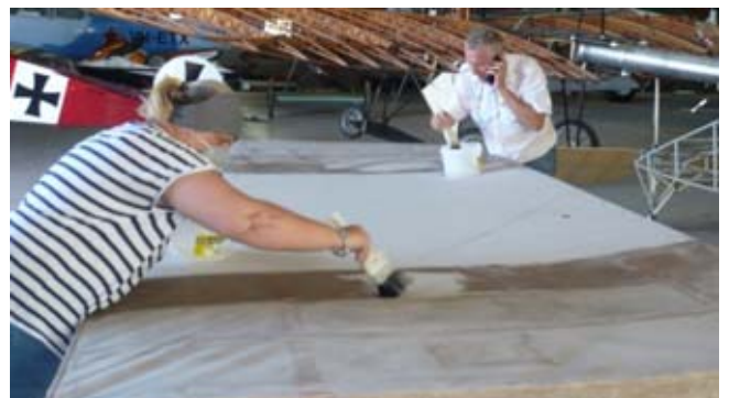
Applying the first layer of dope to the linen surface which instantly sags, before pulling taut.
