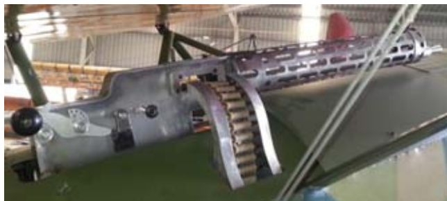
The assembled Spandau machine gun prior to painting, fitted to the Fokker D.VIII with belt and ammo attached.
