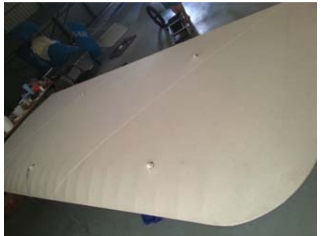
The wing after having been sprayed with water. Note that the fabric was sewn at 45 degrees to the wing.
