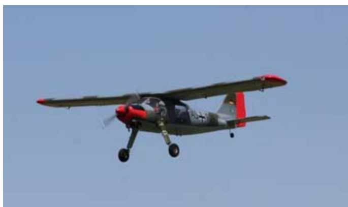
Roly Gaumann's Dornier Do. 27 is an own design spanning 2.2m and powered by a DLE 30cc petrol engine.
