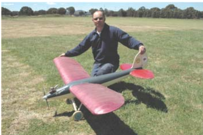
Neal Cator with his Pegasus old timer powered by an Enya 60 four stroke.
