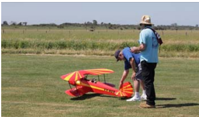
Wally Burston from the Westernport club flew his Stampe SV4. This model is 1/4 scale with a wingspan of 2.1m and is powered by an OS 120 four stroke engine.
