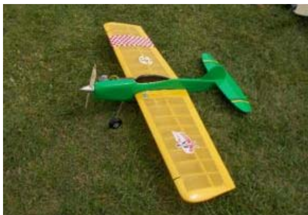
John Goodge presented this new S1. Extra reinforcement at the front end keeps the K&B 40 in check. Beautiful model but you have to hang on tight when it leans out towards the end of the flight.
