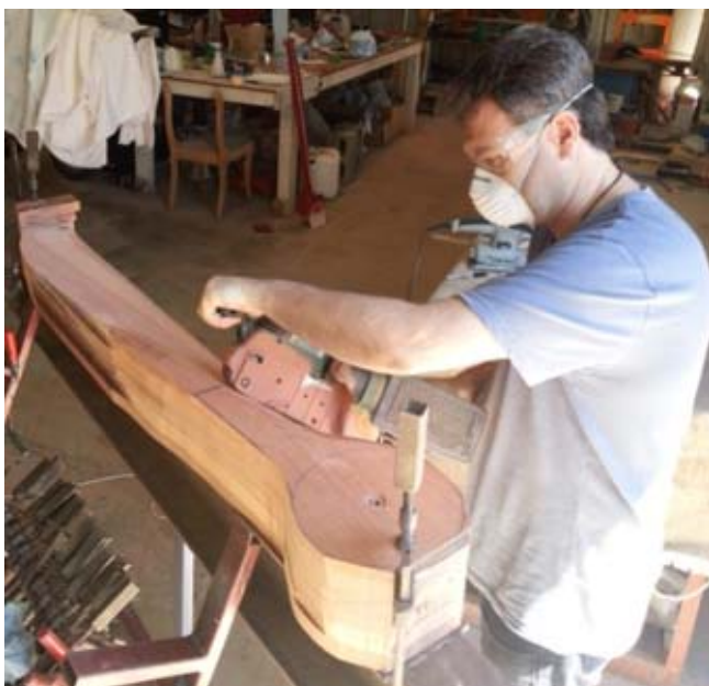
Yours truly sanding the blank Dieter had cut. This half a propeller is used on the cutting machine to make a full propeller with two identical blades
