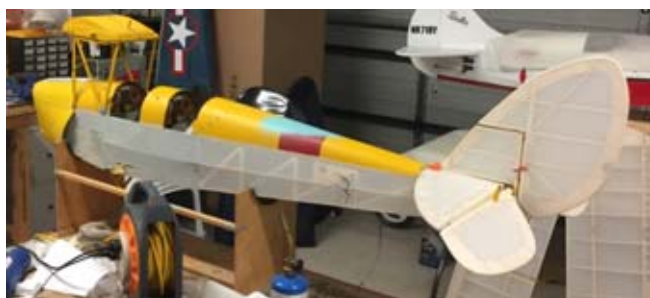
Recovered and with the typical flat spot now showing on the top of the rudder.
