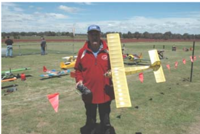
Robert Wilkins with his Tomboy powered by a Taipan 1cc diesel. With a 4.5ml tank the motor runs for 55 sec. and the model has a best flight time of 13min 41sec.
