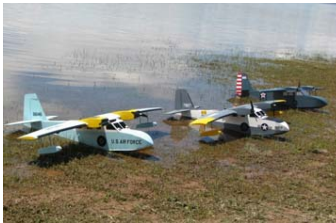
More by Tony Gyoles, these "Puddle XLII" models are based on the Grumman "Widgeon". Constructed from 6mm Depron and electric powered they have a wingspan of 1430mm and are again available from Tony as kits. Owners (from left) are John Nicholas, Tony Gyoles and Mike Guinness.
