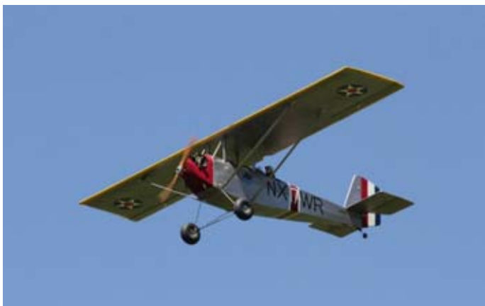
Lew Rodman's Pietenpol Aircamper is 1/3 scale with a wingspan of 2.5m and powered by a TEY 52cc petrol engine.
