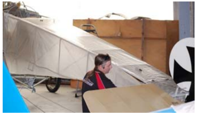
Fitting and cutting the plastic sheet which is then used as a template to cut the linen.
