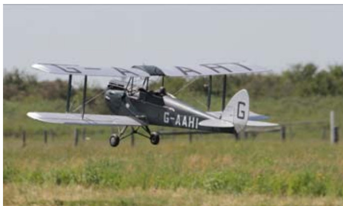
Rob Popelier came from Shepparton with his DH 60 Gypsy Moth. The model is 1/4 scale with a wingspan of 2.3m and is powered by an OS 120 four stroke engine.
