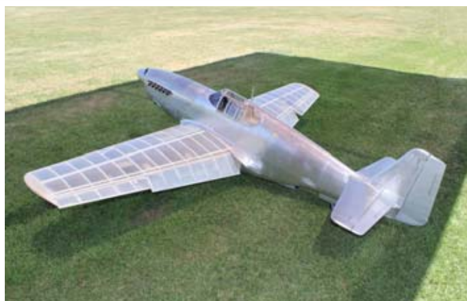
Neil Addicott's P-51 Mustang is built from the Jerry Bates plans and has a wingspan of 2.3m. Powered by a Roto 85cc inline twin the model is covered with aluminium tape.
