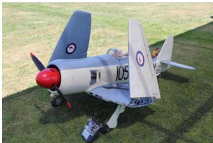
Brian Hutchinson's Hawker Sea Fury is also built from a Jerry Bates plan. Model spans 2.6m and is powered by a 3W 100cc twin cylinder engine.
