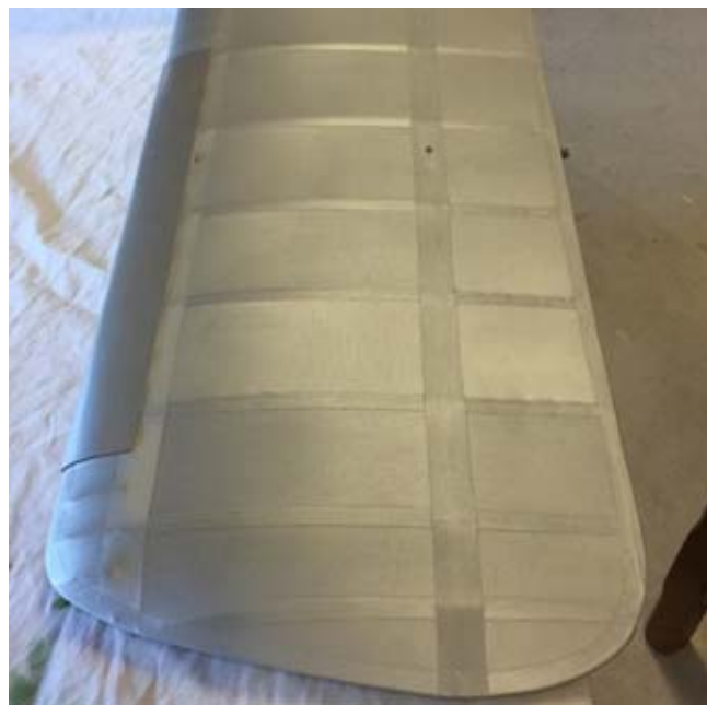
Upper left wing panel recovered with rib stitching and tapes.
