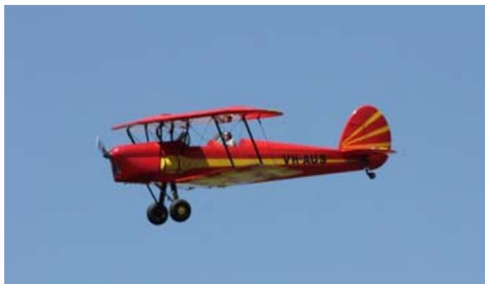
Wally Burston from the Westernport club flew his Stampe SV4. This model is 1/4 scale with a wingspan of 2.1m and is powered by an OS 120 four stroke engine.
