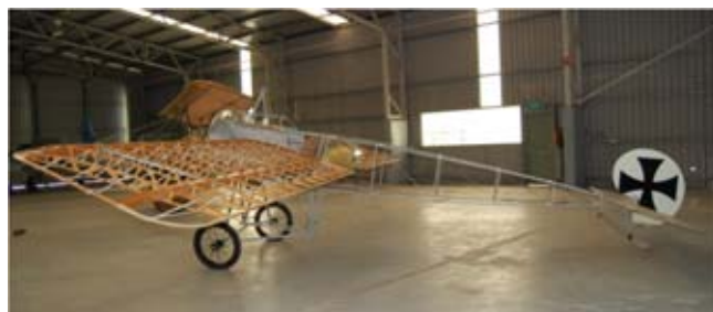
The bare bones of the Achim Engels' reproduction Fokker E.III as it arrived from Germany.
