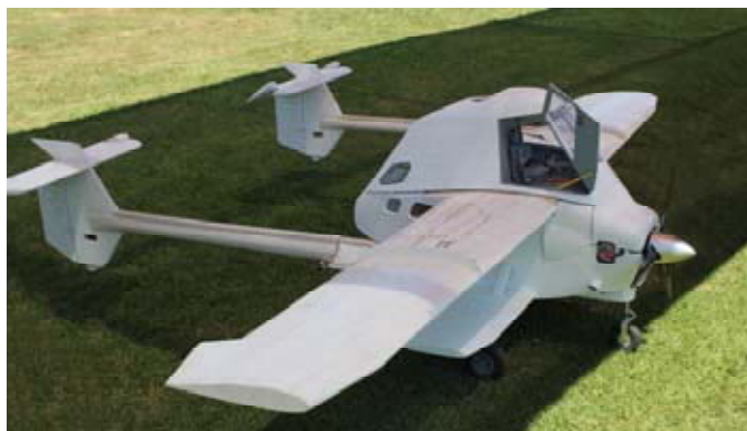
Ray Chivers' Transavia PL-12 Airtruk is nearing completion. Model spans 3.1m and is powered by a DA 70cc petrol engine.
